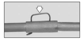
**Rear Flat Tire:** Attach the jack handle extension (D) to the jack handle (E) and then press the clip (arrow) so it engages. Then attach the jack handle (E) with the hook end connected to the u-hook/clevis on the jack (A). Slide the ratchet (F) onto the jack handle extension (D) with the UP mark facing you.
